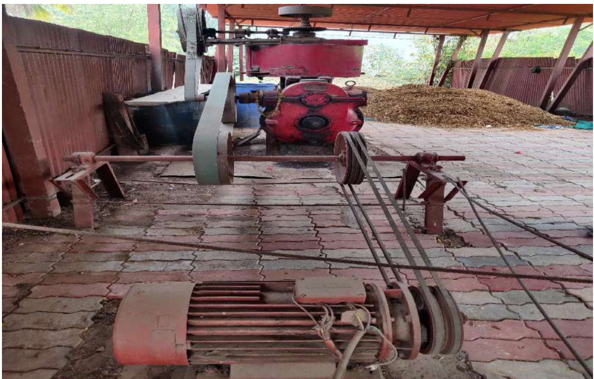
Expeller for Compost Making from Agricultural Waste : Capacity 200 Kg. Per Hour At Israma, Petlad Training / Demonstration Center
