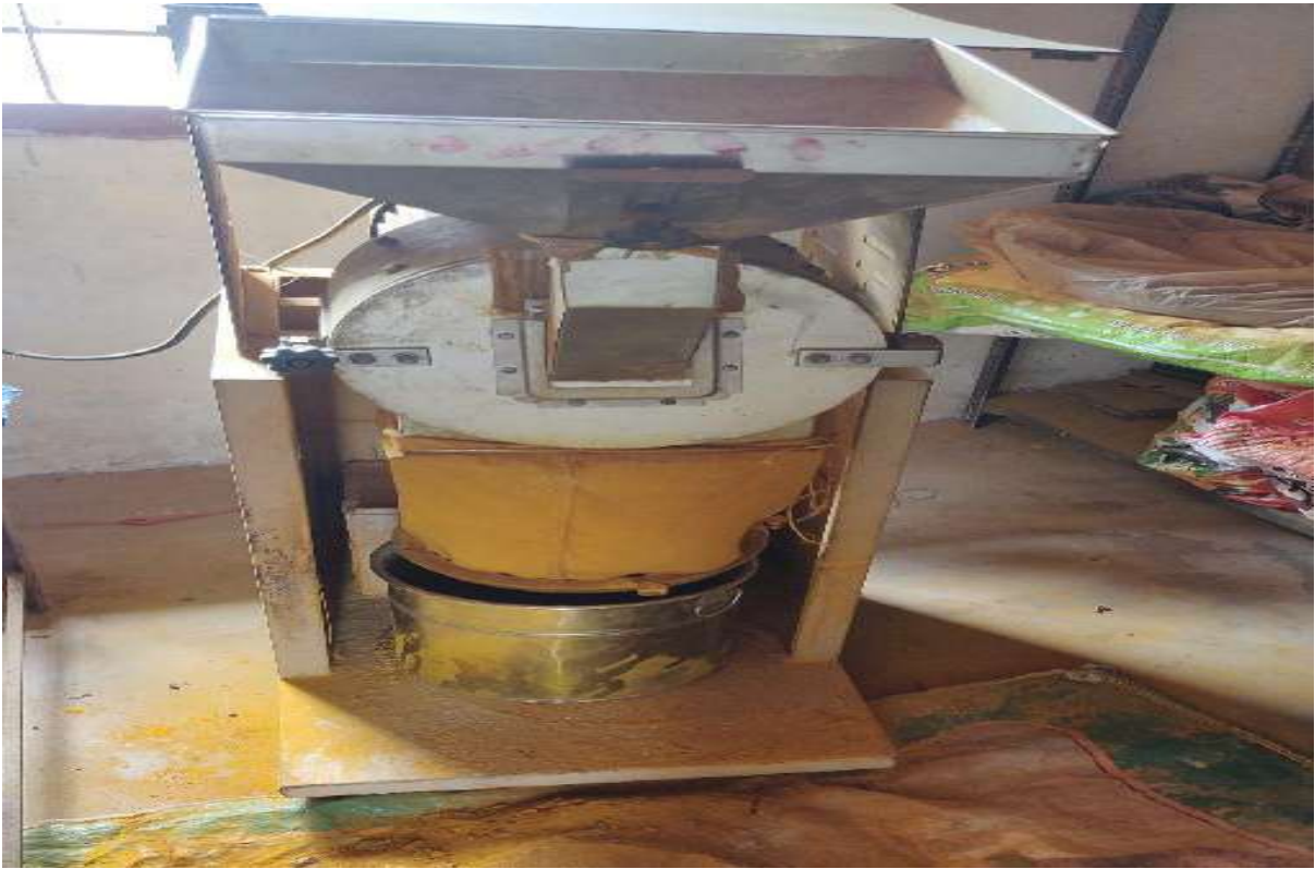
Low Temperature Grinder for Turmeric, Ginger Etc. At Israma, Petlad Training / Demonstration Center
